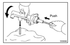
(b) Push in the piston with a screwdriver, and remove the straight pins by turning over the cylinder body.
